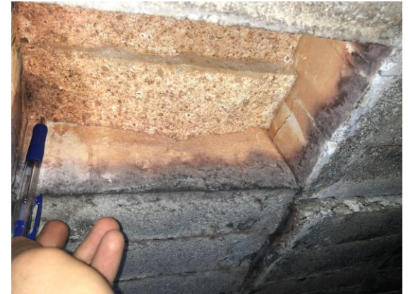
First shutdown post study showing hot face brick failure at the 12 o'clock position
